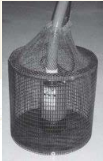
Installation of fish screens
